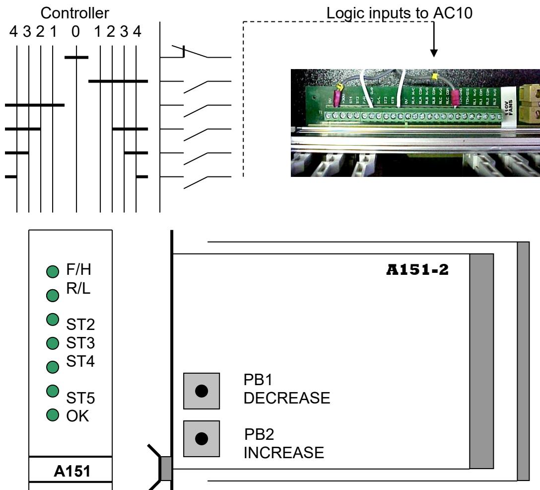
LED's 1 – 5 indicate the direction and speed position of the master controller.
